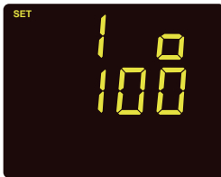
Fig 3-3 Full range shunt setting
