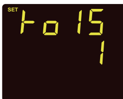
Fig 3-28 RO1 Alarm Inequality Setting
