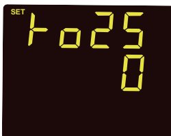
Fig 3-34 RO2 Alarm Inequality Setting
