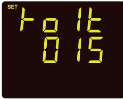
Fig 3-30 RO1 Alarm Delay Setting
