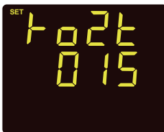
Fig 3-36 RO2 Alarm Delay Setting
