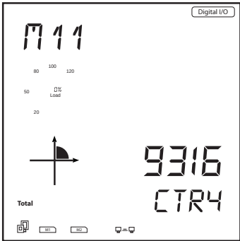
Figure 5-24 Digital Input Pulse Count from Meter's Display
