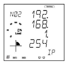
Press 'P' to get to "N03 Subnet Mask". Press 'V/A' to configure the subnet address. The cursor of the first digit will begin to flash. Press the 'H' button to scroll through the digits, press the 'P' or 'E' to change the value of the flashing cursor and press 'V/A' to confirm.
