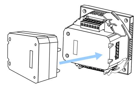
The AXM-WEB2 module is linked to the Acuvim II series meter by a communication plug. Other extended modules such as the IO modules can be linked to the Acuvim II series meter through the AXM-WEB2.
