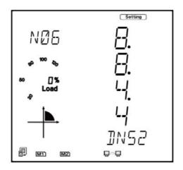
Press 'P' to get to "N07 Modbus Port". Press 'V/A' to configure the Modbus Port. The cursor of the first digit will begin to flash. Press the 'H' button to scroll through the digits, press the 'P' or 'E' to change the value of the flashing cursor and press 'V/A' to confirm.
