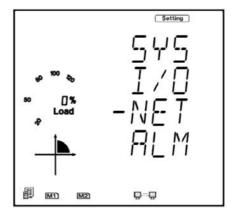
The first page of the NET Settings will be the N01 DHCP setting. By default this is configured to Manual. Setting this configuration to Auto will allow the router to assign the meter with an IP address, whiles Manual will allow the user to configure the IP address. Press the 'V/A' button to enter edit mode. Press 'P' or 'E' to change the setting and press 'V/A' to confirm.
