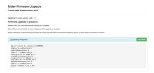
When the firmware update is complete, the module will reboot. The rebooting process will take 5 to 10 minutes to complete.
