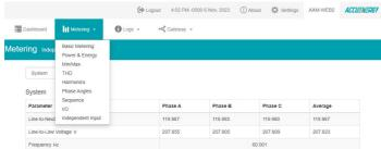
When enabling the independent channel feature, the independent input will appear in the dropdown menu under metering. Users can view the corresponding values:
