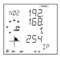
Press 'P' to get to "N03 Subnet Mask". Press 'V/A' to configure the subnet address. The cursor
