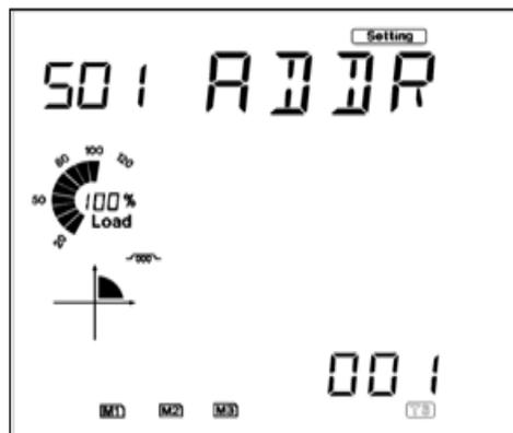
Figure 2- Device address setting
