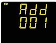
Figure 3-19 Communication address setup
