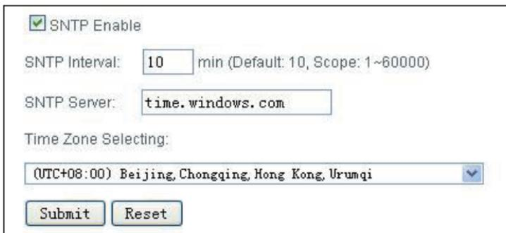
The screenshot shows a configuration window for SNTP settings. It includes a checked checkbox for 'SNTP Enable', a text input for 'SNTP Interval' set to '10' with a unit of 'min' and a default note '(Default: 10, Scope: 1~60000)', a text input for 'SNTP Server' set to 'time.windows.com', a 'Time Zone Selecting:' label, and a dropdown menu currently showing '(UTC+08:00) Beijing, Chongqing, Hong Kong, Urumqi'. At the bottom are 'Submit' and 'Reset' buttons.
