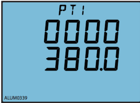
Fig.3-42 PT primary side ratio setting
