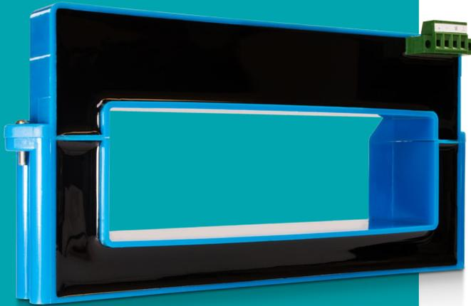
The HAB Series Hall effect DC current sensor is designed to measure up to 5000A of DC current with 0.5% accuracy. Designed to adapt, the HAB is available with either 4-20mA or 0-5V output and as either a uni-directional or bi-directional device for broad compatibility. Suited for existing applications, the split-core design can be installed without wire or cable disconnection.
